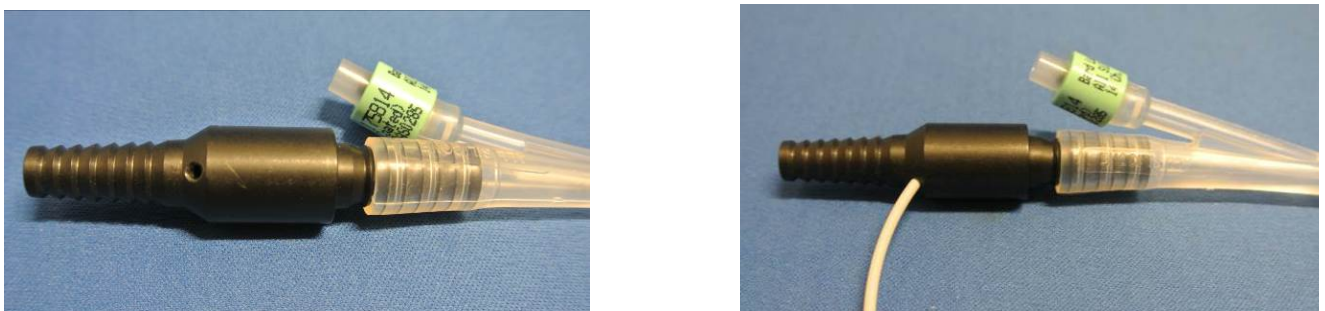
Figure 9: Details of the optical fibre insertion at the distal end of the Foley catheter.
