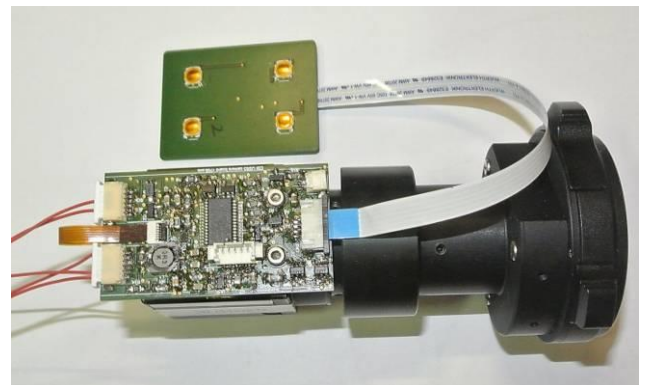
Figure 1: The completed programmable imaging lens, its drive circuit and control switches, fitted around a small camera.
