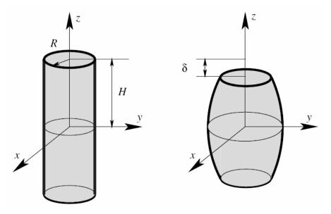
(i) Introduce the barrelling function as the ratio between the deformed external radius at height *z* and the initial radius, f(z/H) = R'(z)/R. Show that the displacement field (u, v, w) with respect to cylindrical polar coordinates  $(r, \theta, z)$  given by  $u = \frac{\delta}{H} v \frac{r}{R} f(z/H)$ , v = 0,  $w = -\frac{\delta}{H} z$  is kinematically admissible.
