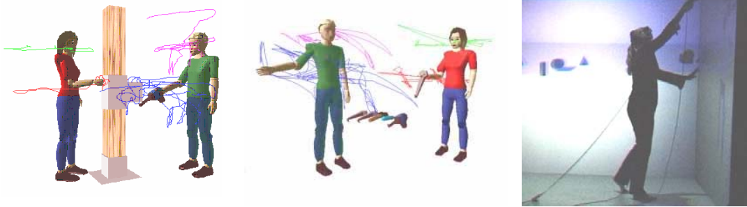
Figure 4: Left: Two participants fix a bracket to an upright in the Gazebo task. The tracks indicate recent head and hand moves Middle: When planning a task the instructor (on the left) moves much more frequently than the student (on the right). Right: A participant manipulates an object whilst making sure that they do not touch the physical wall of the IPT.
