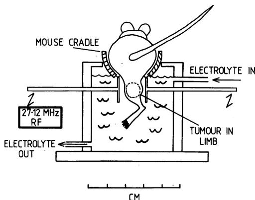
FIG. 1.—The RF heating system.
