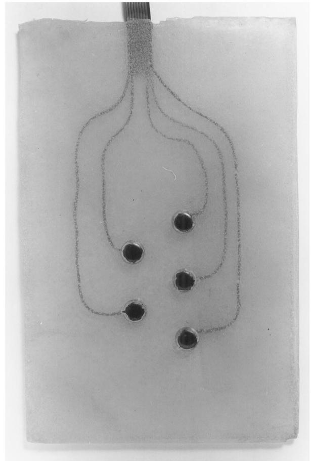
Fig. 1. Apparatus employed to record skin conductance.
