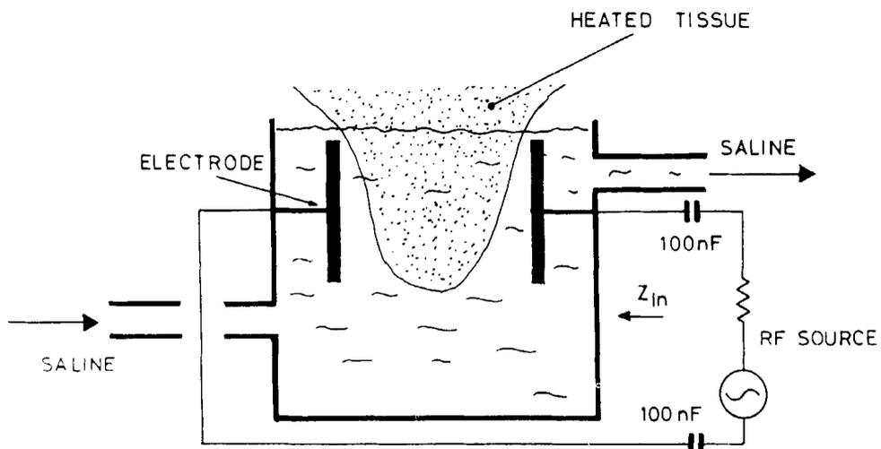
Figure 1. Outline of the heating jig used, which presents approximately a  $100\Omega$  impedance, ( $Z_{in}$ ), to the RF source. The  $100\text{ nF}$  coupling capacitors present a negligible reactance at RF but limit mains earth loop currents set up through the RF source, the saline flow system thermostat and the mains supply.
