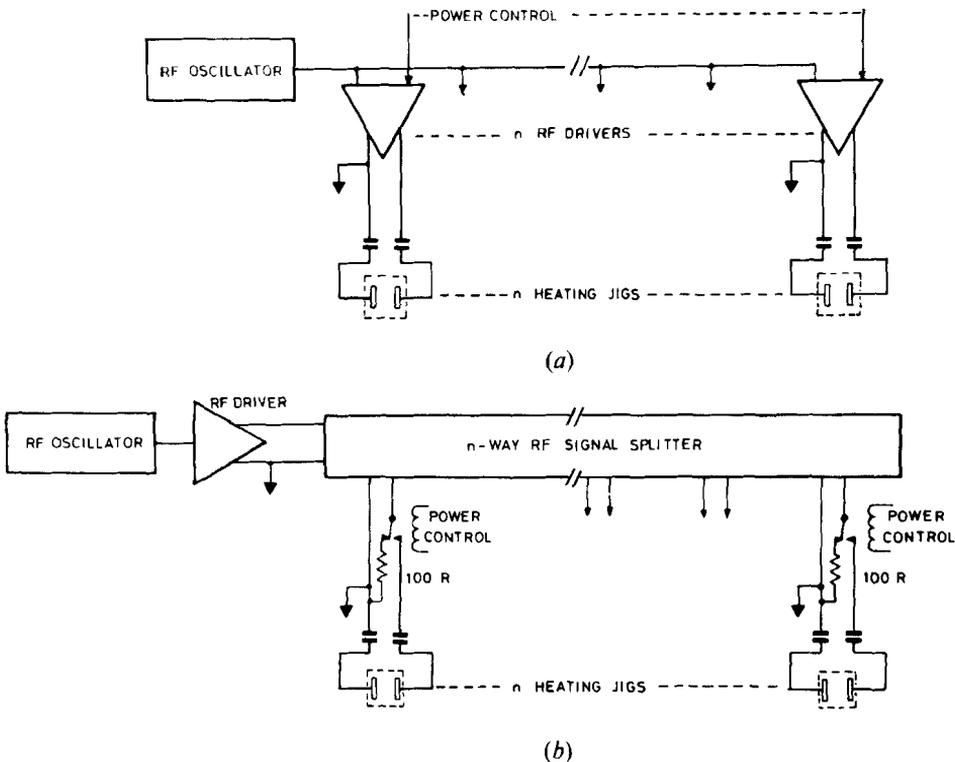
Figure 2. Simultaneous heating of a number of jigs can be performed using a number of drivers, each independently controlled as in (a) or by splitting the output of one driver, as in (b). For the latter case, the splitter output can be switched between the jig and a dummy load; the mark-space ratio of the relay operation therefore controls average power delivered to the jig.
