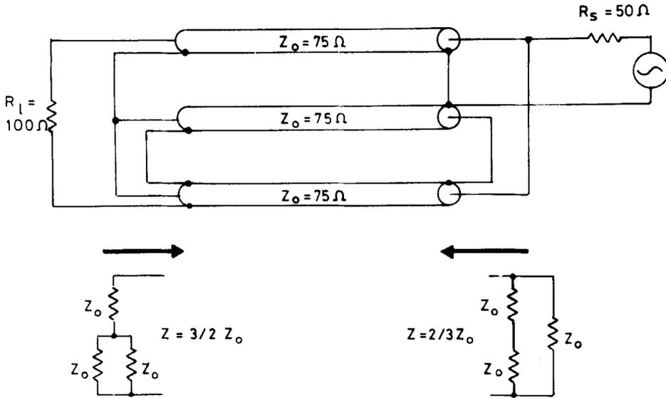
Figure 6. A broadband transmission-line 2:1 impedance ratio transformer. The transmission lines of impedance  $Z_0$  at the input and output of the transformer are connected to produce impedances of  $3Z_0/2$  and  $2Z_0/3$ . The lines are wound on MM625/T1 cores,  $3 \times 3$  turns of RG59 cable. A bandwidth of 3–30 MHz and power handling of  $>200$  W can be achieved.
