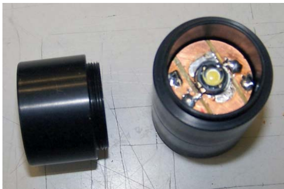
Figure 3: The collimated LED source in practice. The left image shows the LED soldered to the printed circuit board, with the aspheric lens holder to the side. The right image shows copper stud mounting screw and connections to the mini-DIN socket
