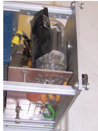
Figure 3: A successful attempt to produce an ultra-fast PMT detector at low cost.
