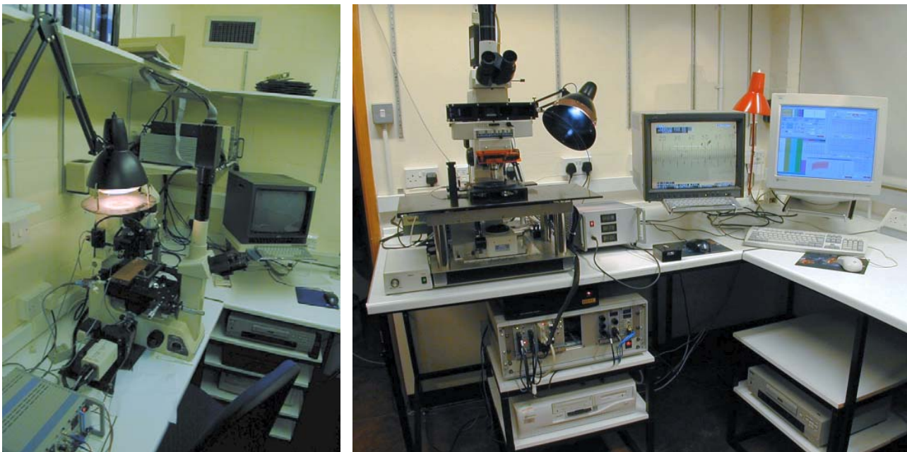
Figure 1: Two of GCI's intravital microscopes. Left: the original system based on an inverted microscope. Right: system based on an upright microscope and featuring a large stage/sample platform.
