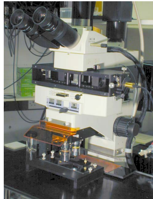
Figure 6: Practical realisation of the optical system depicted in Figure 5, constructed in an assembly placed above the fluorescence cube block and below the eyepieces/camera ports.
