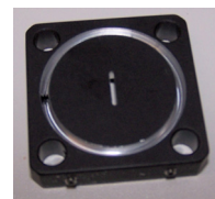
Figure 3. A galvanometer scanner lens relay system constructed from Thorlabs C6W cubes on the ends, CP02 / CP02T cage plates and SM1L05 lens tubes. A custom machined CP01 plate in the centre forms a slit and isolates the X and Y scanning systems. Plastic tubes (Thorlabs SC1L24) are held in the slit assembly and in dummy lens tubes (not shown in the SolidWorks model)
