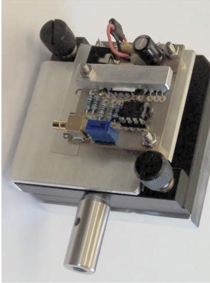
Here is an even simpler, open-loop version of the optical delay line, with just the driver and no sensor arrangement, mounted on a 2" optical mirror mount.
