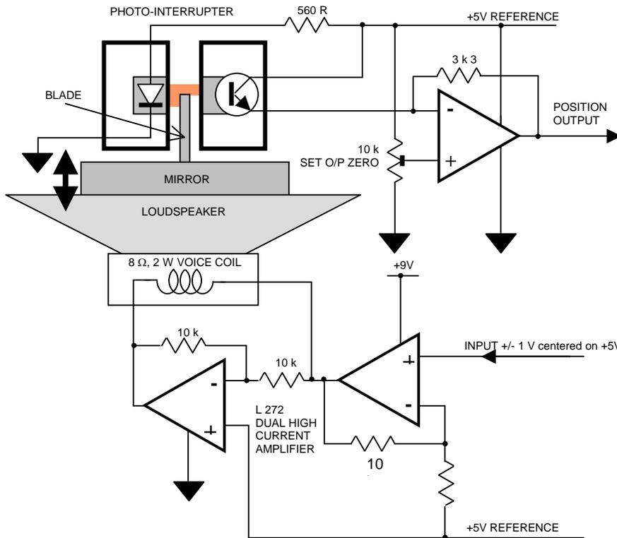
The control electronics may be modified such that the position output can be used to ‘close the loop’ and ensure that the loudspeaker responds to the input in a consistent, frequency independent manner. Although sinewave excitation is primarily employed, there may be instances where other frequencies may be present, e.g. when driving the system with triangular waveforms.
