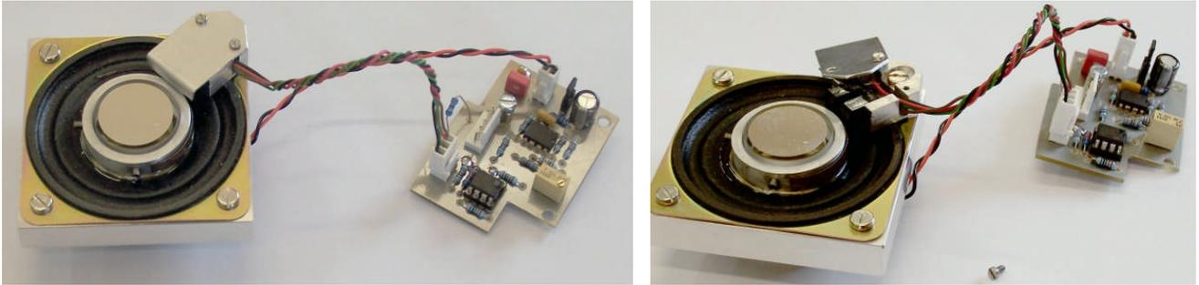
How the voice-coil optical delay line is implemented in practice: the loudspeaker and sensor assembly form a single unit which is connected to a small printed circuit board with short wires. These subassemblies are then mounted on a standard 2" optical mirror mount.
