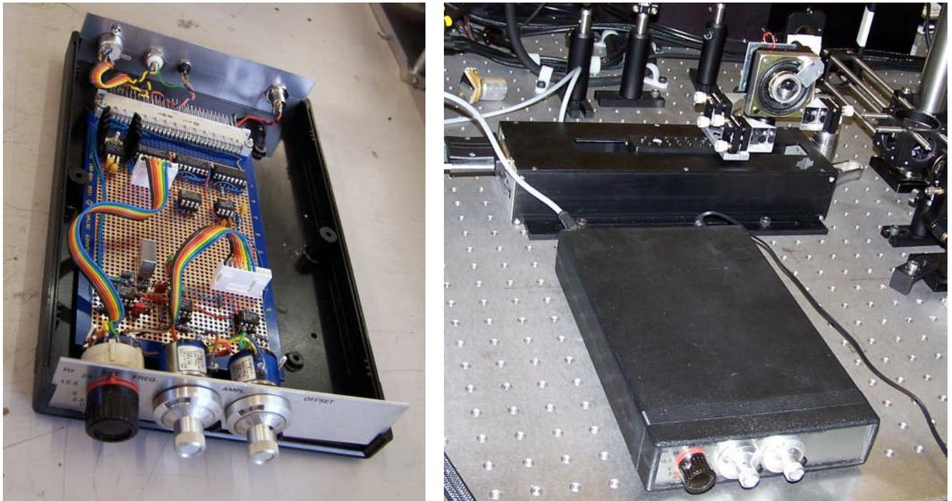
The sine-wave generator used to drive the optical delay line (left) and the complete arrangement in use (right).
