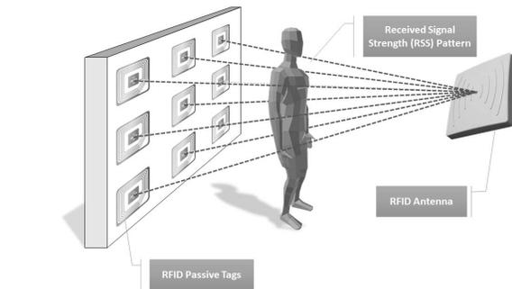
Fig. 1. Proposed lightweight setup: a person does not need to wear any devices and performs different postures between the wall and an RFID antenna. The postures can be recognized by analyzing the corresponding sensing data collected by the RFID reader.
