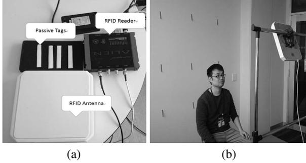
Fig. 6. In (a), we show the devices used in our experiment, including 1 RFID reader (Alien 9900+), 1 Alien Circular Antenna and a collection of Alien Squig RFID Inlay passive tags. In (b), we show the experimental layout in our implementation, one subject is sitting between tag array and antenna and performing predefined postures.
