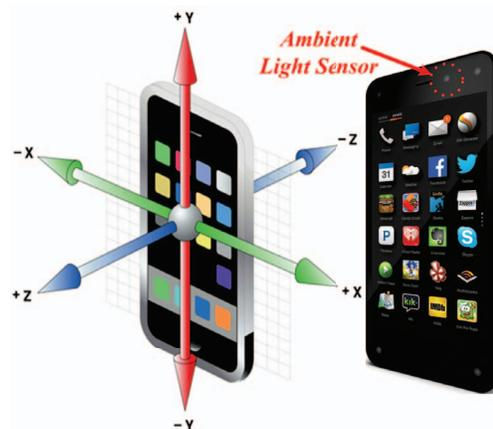
Fig. 2: Three-axis accelerometer and light sensor
