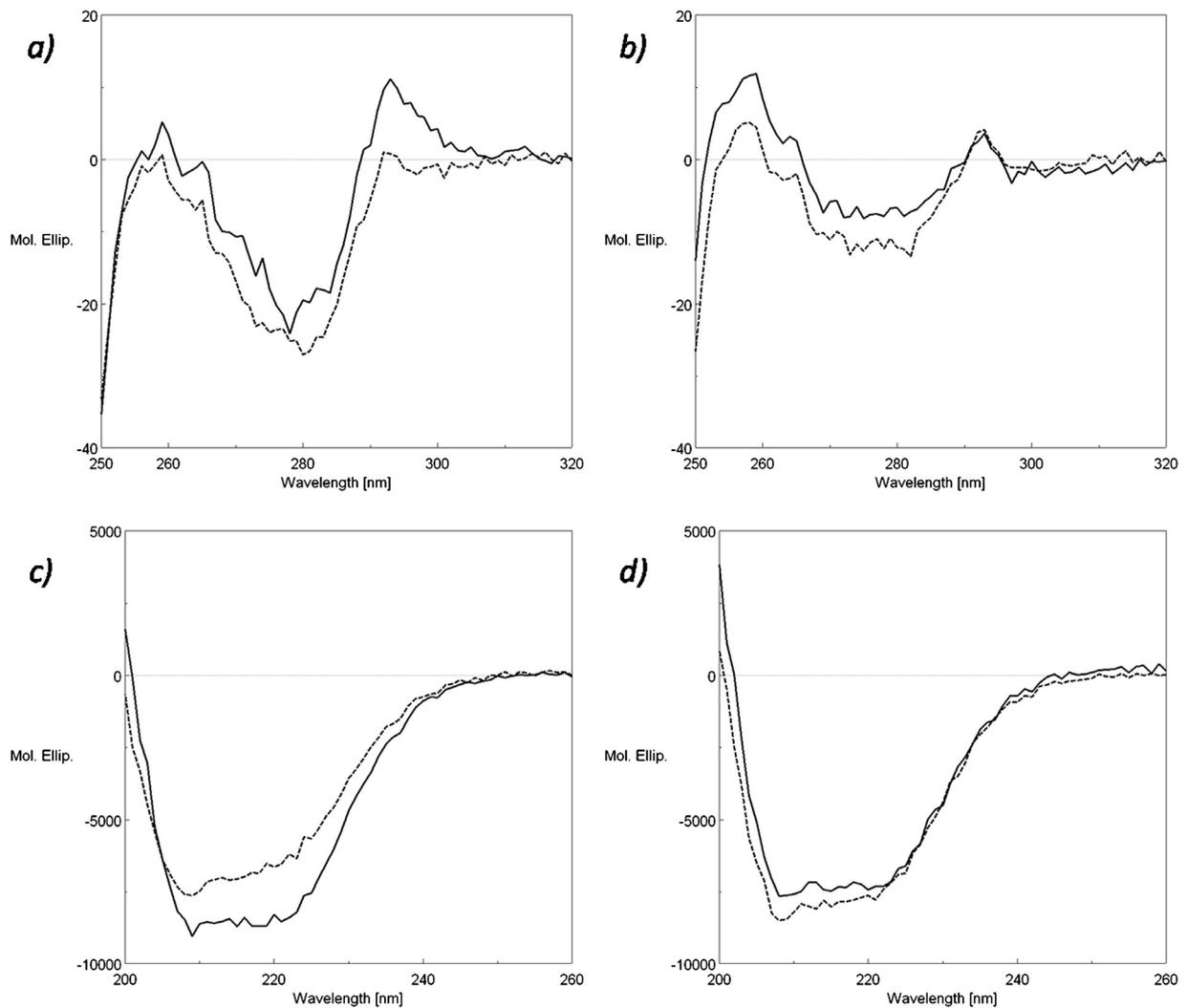
**Fig. 3.** CD spectra of carrier proteins (solid line) and their glycosylated MenA conjugate (dashed line); (a) near-UV and (c) far-UV spectra of CRM<sub>197</sub> conjugates; (b) near-UV and (d) far-UV spectra of DT-K51E/E148K conjugates. The buffer blank was subtracted from the baseline of all spectra. Mol. Ellip. = molar ellipticity, expressed in degree  $\times$  cm<sup>2</sup>  $\times$  dmol<sup>-1</sup>.
