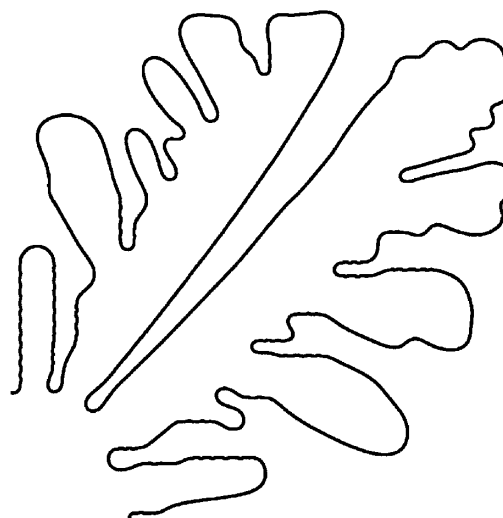
FIG. 1. Example phase-field calculation showing the morphology of a dendrite subject to kinetically induced tip splitting (after Ref. [14]).
