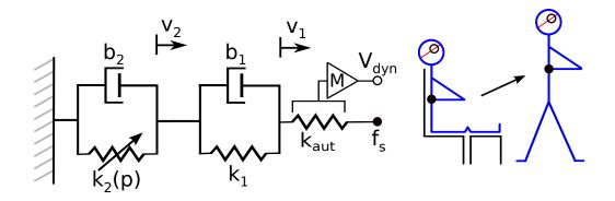
**Figure 2**: Mechanical analog used for predicting  $V_{dyn}$
