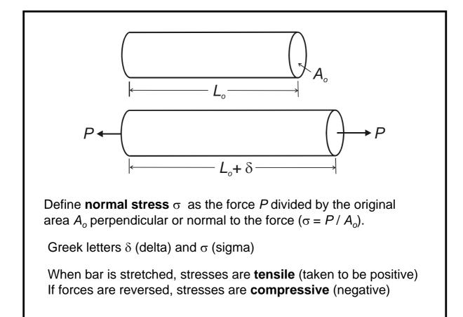
**Example**: Prismatic bar has a circular cross-section with diameter d = 50 mm and an axial tensile load P = 10 kN. Find the normal stress.
