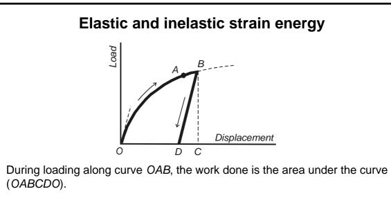
If loading is past the elastic limit *A*, the bar will unload along line *BD*, with permanent elongation *OD* remaining.
