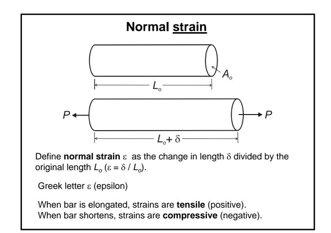
**Example**: Prismatic bar has length  $L_o = 2.0$  m. A tensile load is applied which causes the bar to extend by  $\delta = 1.4$  mm. Find the normal strain.
