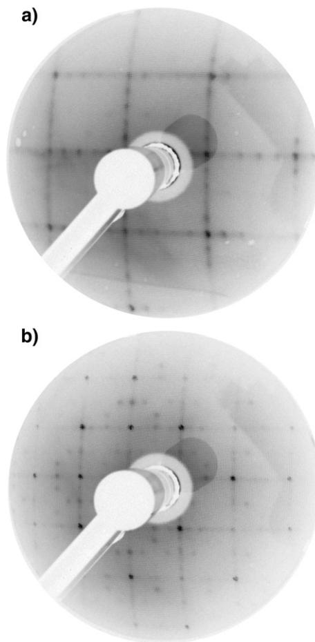
**Fig. 4.** LEED patterns of a sample surface with 3.50 MLs of Ti deposition, taken at electron beam energies of 63 eV and 147 eV, showing the (5 × 1) reconstruction in (a), and mixed (5 × 1) and c(4 × 2) reconstructions in (b).
