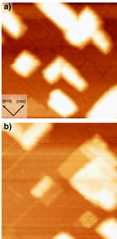
**Fig. 3.** (a) Depositing 3.50 MLs of Ti and post-annealing gives rise to a higher coverage of bright islands on the nanoline-covered SrTiO<sub>3</sub> surface. (Image size: 44 × 44 nm<sup>2</sup>, V<sub>s</sub> = 0.85 V, I<sub>t</sub> = 0.08 nA). (b) Longer annealing time allows the observation of a row structure on the islands (Image size: 45 × 45 nm<sup>2</sup>, V<sub>s</sub> = 0.83 V, I<sub>t</sub> = 0.20 nA).
