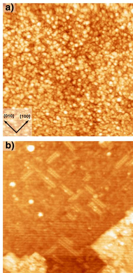
**Fig. 7.** STM images showing (a) a disordered surface following Ba and Ti deposition on a degassed SrTiO<sub>3</sub> substrate (Image size: 100 × 100 nm<sup>2</sup>, V<sub>s</sub> = 1.07 V, I<sub>t</sub> = 0.10 nA); (b) dilines and bright BaO nanoparticles on the c(4 × 2)-reconstructed SrTiO<sub>3</sub>(001) surface after UHV annealing of the surface at 800 °C for 1.5 h (Image size: 50 × 50 nm<sup>2</sup>, V<sub>s</sub> = 0.78 V, I<sub>t</sub> = 0.20 nA).
