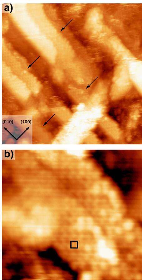
**Fig. 6.** STM images showing (a) a locally ordered structure indicated by arrows following Ba deposition onto a sputtered SrTiO<sub>3</sub> substrate surface with post-annealing (Image size: 46 × 46 nm<sup>2</sup>, V<sub>s</sub> = 1.00 V, I<sub>t</sub> = 0.20 nA); (b) details of the ordered structure with a unit cell indicated by the square, enlarged from an image taken from another area on the surface (Image size: 14 × 13 nm<sup>2</sup>, V<sub>s</sub> = 1.28 V, I<sub>t</sub> = 0.20 nA).
