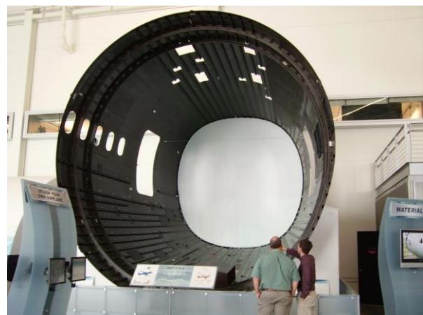
A cured 787 fuselage barrel section
