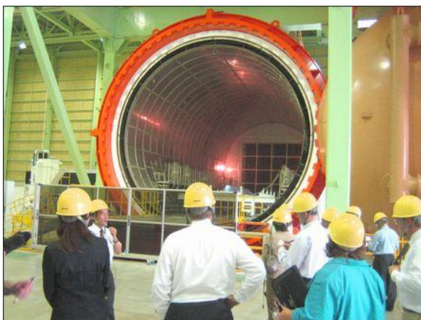
The 787 forward fuselage composite barrel autoclave at Kawasaki, Nagoya, Japan. Source: James Wallace/Seattle Post-Intelligencer
