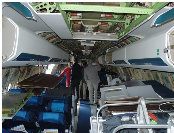
Figure 13. The cabin of a Boeing 757 during parting-out
