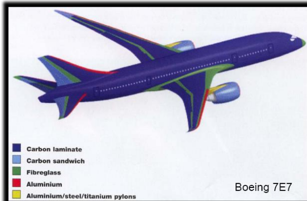
Figure 11. Composite use in the Boeing 787
