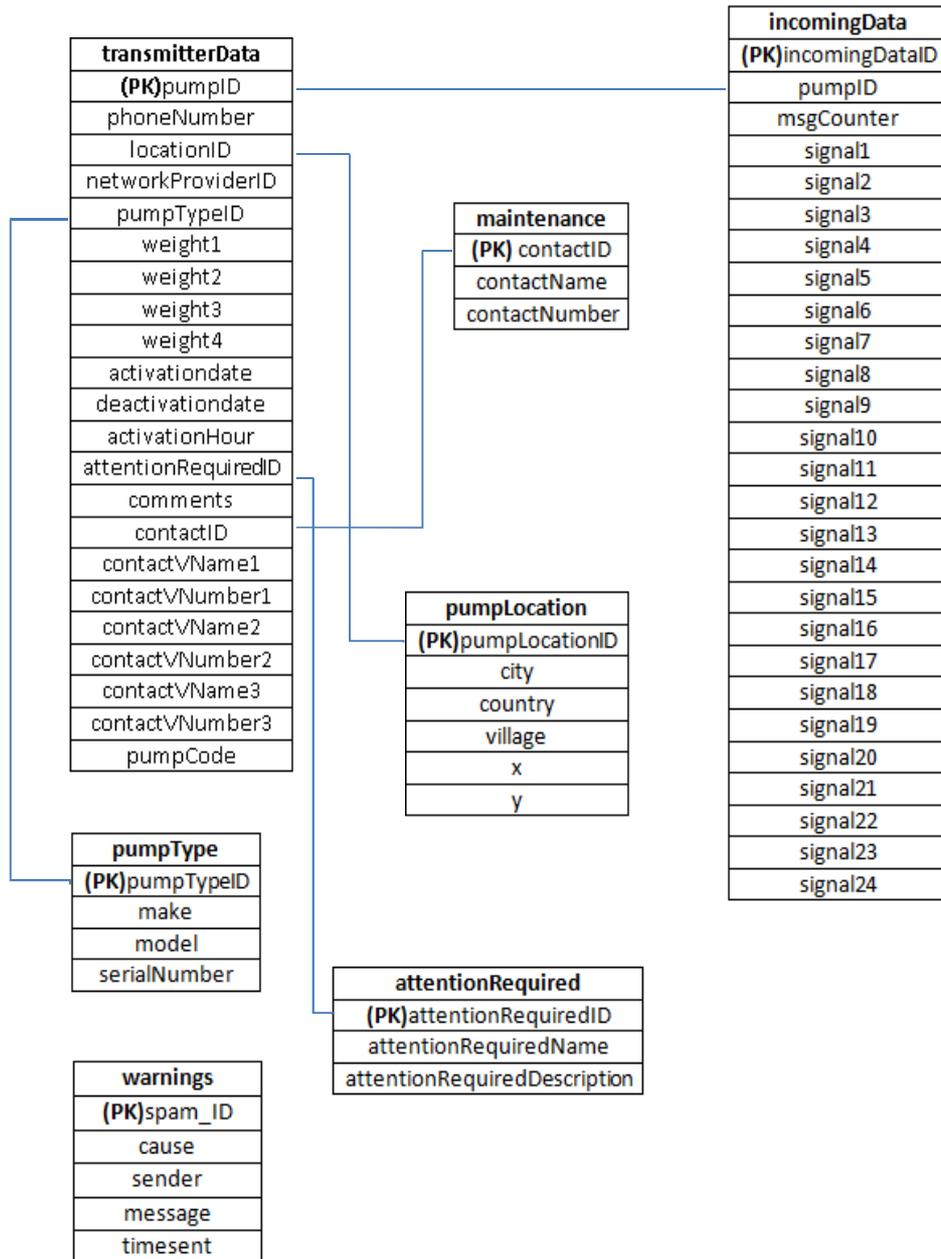
**Figure 9: Relational database structure used to store the incoming data transmitted by SMS from the pump to the server. The database holds additional information relative to the individual pumps.**
