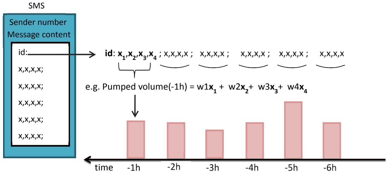
**Figure 2: SMS structure and its relation to water consumption.** Each SMS contains a timestamp, sender number, message number and a series of measurements ( $x$ ). Water consumption is obtained when the latter are multiplied by pump specific weights ( $w$ ). Note that the  $w$  coefficients are stored in the central database and not in the individual SMS.
