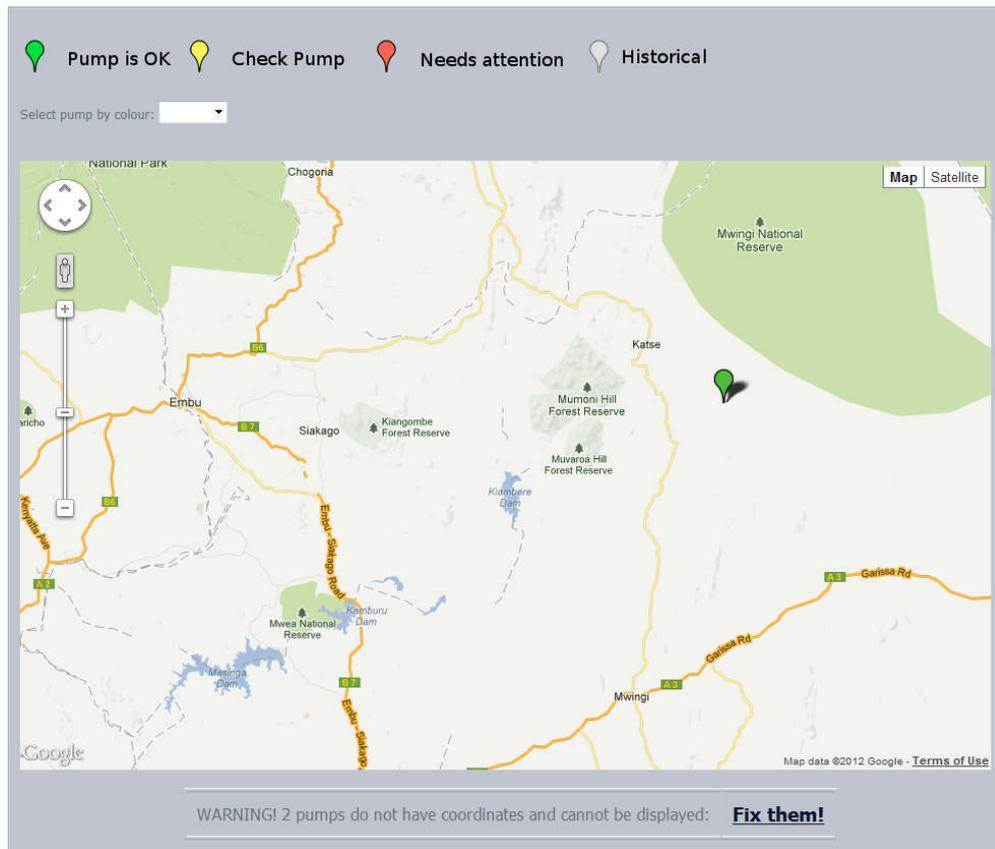
**Figure 4: Transmitter locations interface using Google Maps with colour coding to indicate pump status. Transmitters can be filtered by their status to identify issues rapidly. A dialogue box at the bottom of the map ensures that the user is aware of transmitters with missing geographical information.**
