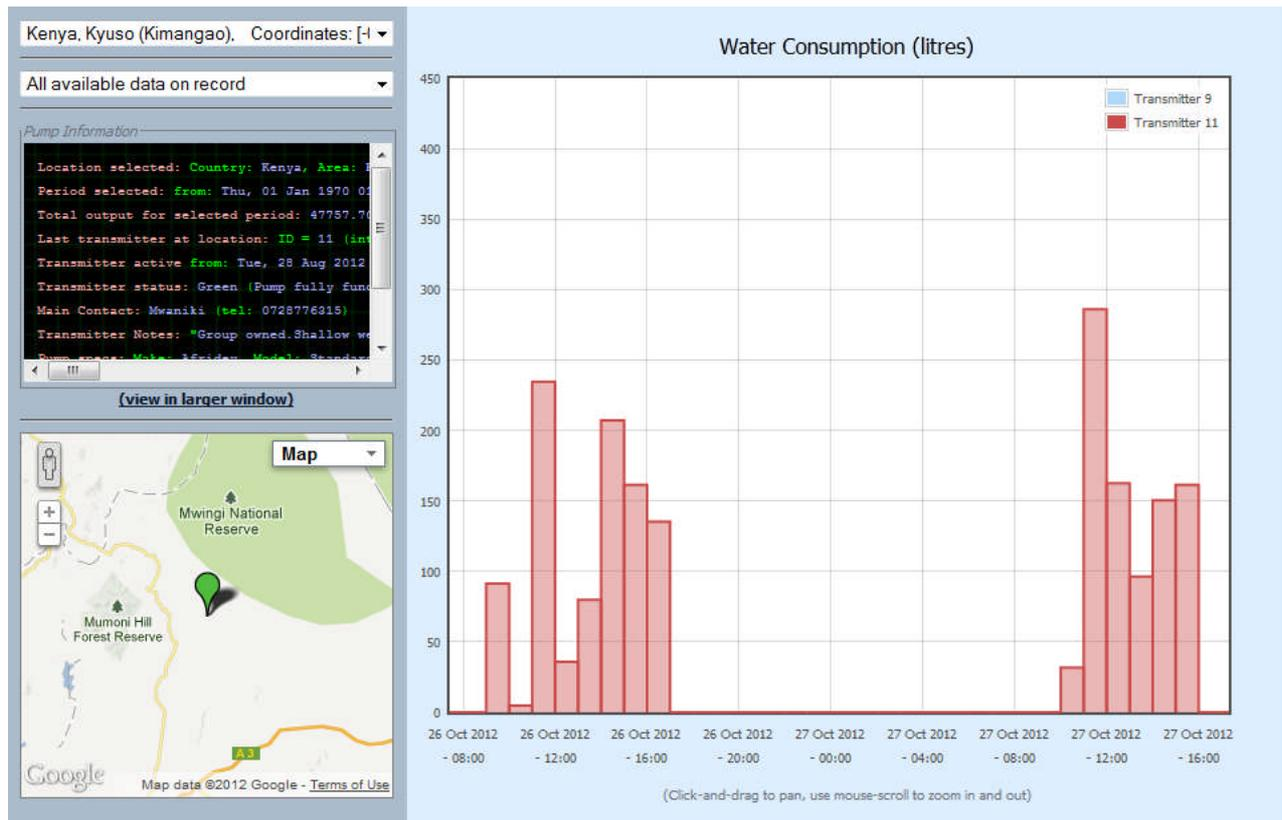
**Figure 5: User interface for visualising estimated water consumption and other useful statistics processed from incoming WDT data. Top left panel: pump and time period selection menus. Middle left panel: useful information is displayed for the given pump. Bottom left panel: mini-map interface showing the location of the pump selected. Right panel: Graphs of water consumption in litres as estimated from WDT data with hourly resolution.**
