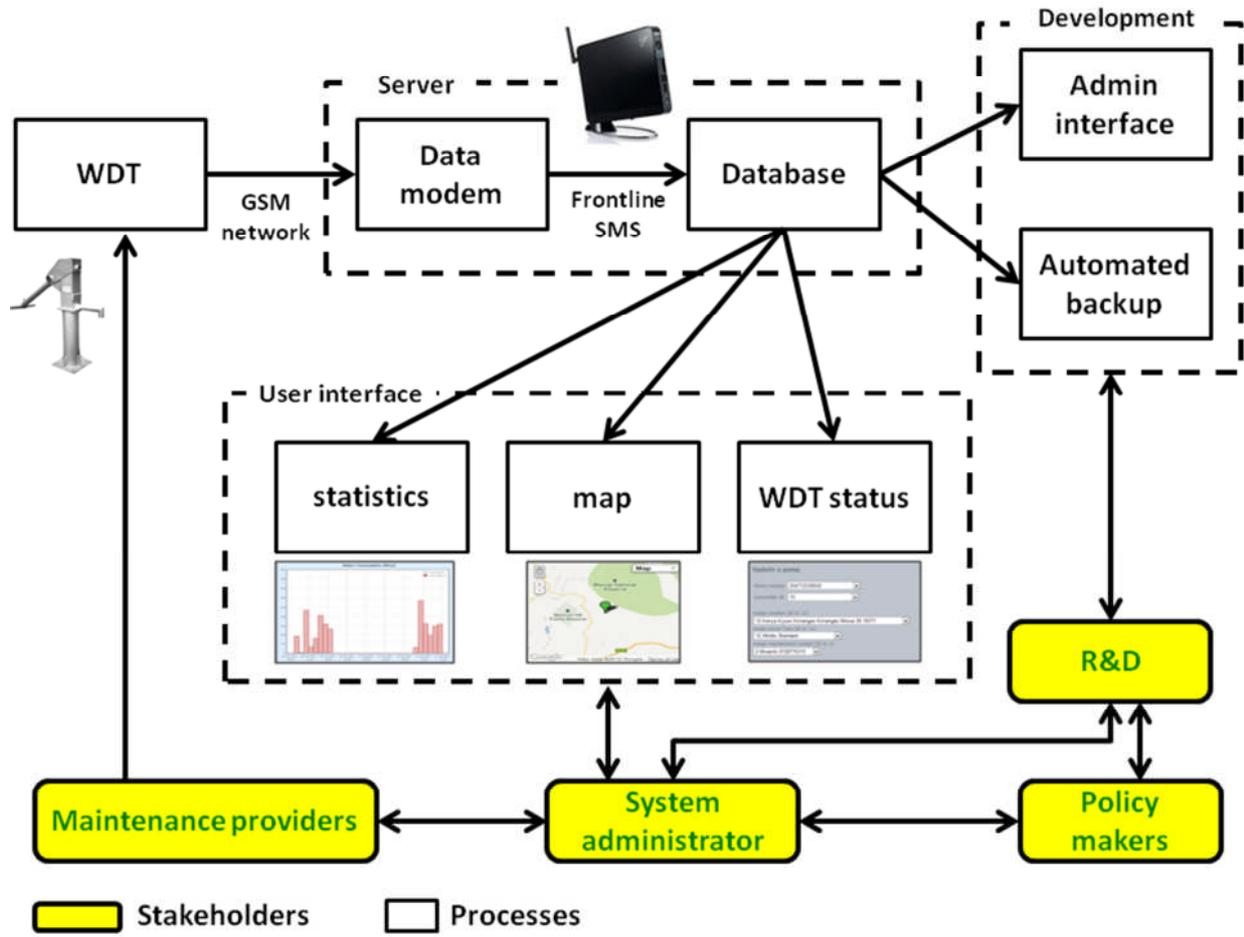
**Figure 1. Architecture design of the system: information about pump usage is acquired via the Waterpoint Data Transmitter (WDT) and transmitted via GSM to a centralised SMS server where information is stored in a database. Stakeholders can access the data via a web interface and manage the monitored pumps via a project-tailored user interface. The research and development (R&D) team has access to its own administration interface.**
