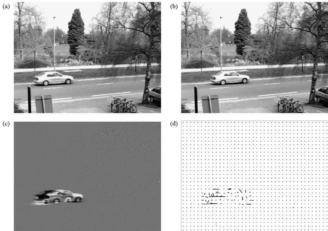
**Fig. 2.** A realistic example of calculating velocity vectors using the optical flow algorithm. (a) Image frame at time  $t$ . (b) Image frame at time  $t + 1$ . (c) Difference between (a) and (b). (d) Velocity vectors.
