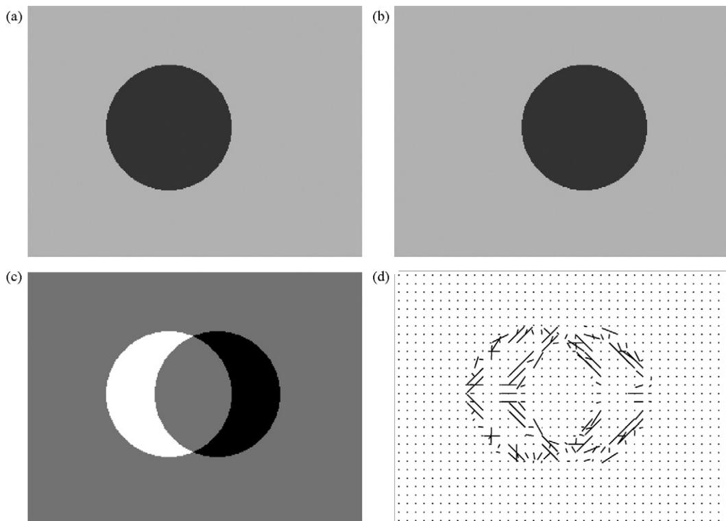
Fig. 1. A diagrammatic example of calculating velocity vectors using the optical flow algorithm. (a) Image frame at time  $t$ . (b) Image frame at time  $t+1$ . (c) Difference between (a) and (b). (d) Velocity vectors.
