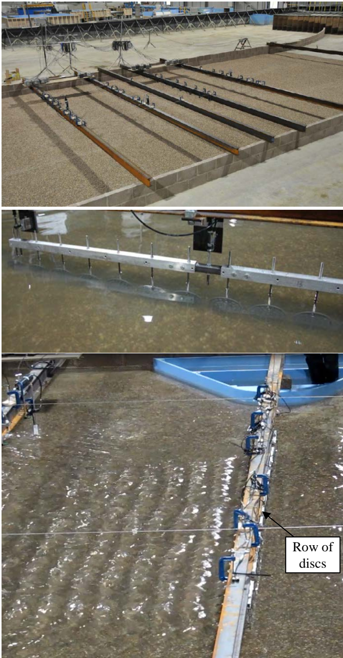
Fig. 2 (Top) Tidal channel, including support beams to mount measurement devices. (Middle) Strip of porous discs. Load cells are also shown. (Bottom) Flow (from right) behind the discs in a headland configuration experiment.
