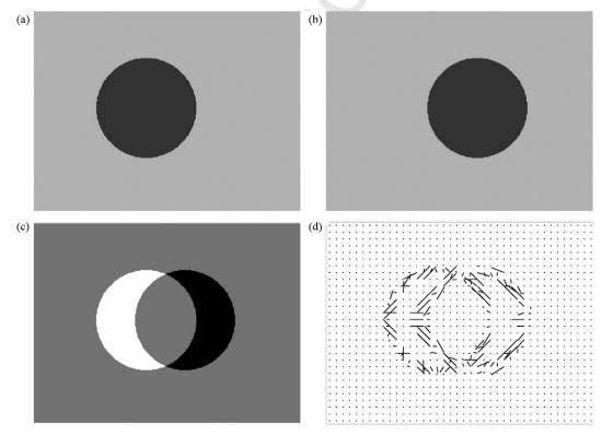
**Fig. 1.** A diagrammatic example of calculating velocity vectors using the optical flow algorithm. (a) Image frame at time  $t_{A}^{(b)}$  Image frame at time  $t_{A}^{(b)}$  (b) Image frame at time  $t_{A}^{(b)}$  (c) Difference between (a) and (b). (d) Velocity vectors.
