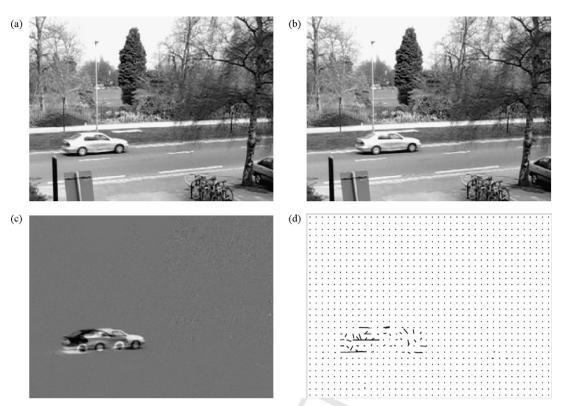
**Fig. 2.** A realistic example of calculating velocity vectors using the optical flow algorithm. (a) Image frame at time  $t_{A}$  (b) Image frame at time  $t_{A}$  (c) Difference between (a) and (b). (d) Velocity vectors.
