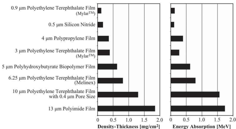
**Fig. 3.** The left chart shows the density-thickness of a selection of substrates. The right chart shows the energy absorption of substrates measured by placing various materials at the output of the microbeam. The input energy of  ${}^3\text{He}^{2+}$  particles to the substrates was 3.85 MeV.
