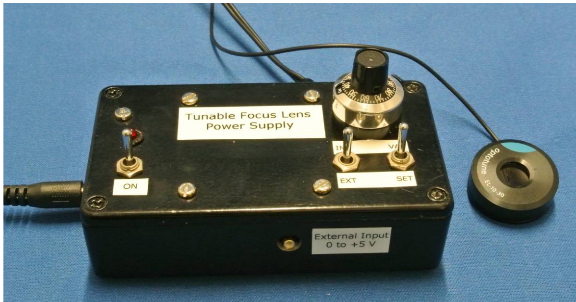
Figure 6: The completed focus-tunable lens constant current power supply: on-off switch on the left, input selection switches on the right and the modulation input socket is just visible on the case side. The power supply input jack is also on the left, while the lens output jack is ‘behind’.
