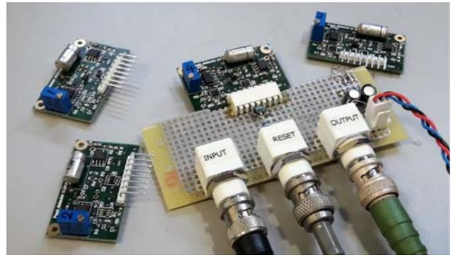
Figure 7: Arrangement used to test the peak detectors. Two 10  $\mu$ F electrolytics decouple the power rails while a 470  $\Omega$  resistor and a small Zener protect the reset input from overzealous pulse generator settings.
