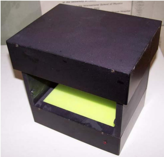
Figure 3: The Mk2 colony counter hardware, based on the principles as the Mk1 version, but providing a larger working area.
