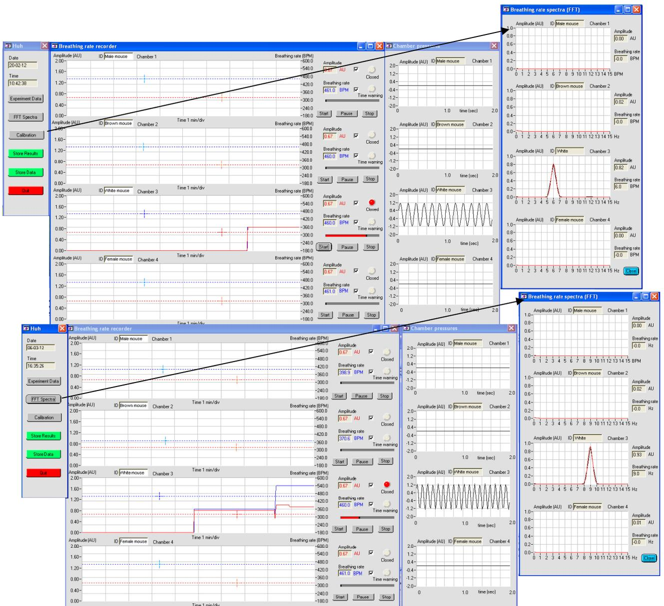
Figure 8: The host GUIs showing the chamber pressure signals and the FFT spectra. In these examples 6.00 Hz (upper panels) and 9.00 Hz (lower panels) sinusoidal signals are fed to the calibration device shown in Figure 2. Although FFT abscissa is scaled in Hz, the chart recorder ordinates are scaled in the more ‘convenient’ units of breaths per minute, ‘bpm’.
