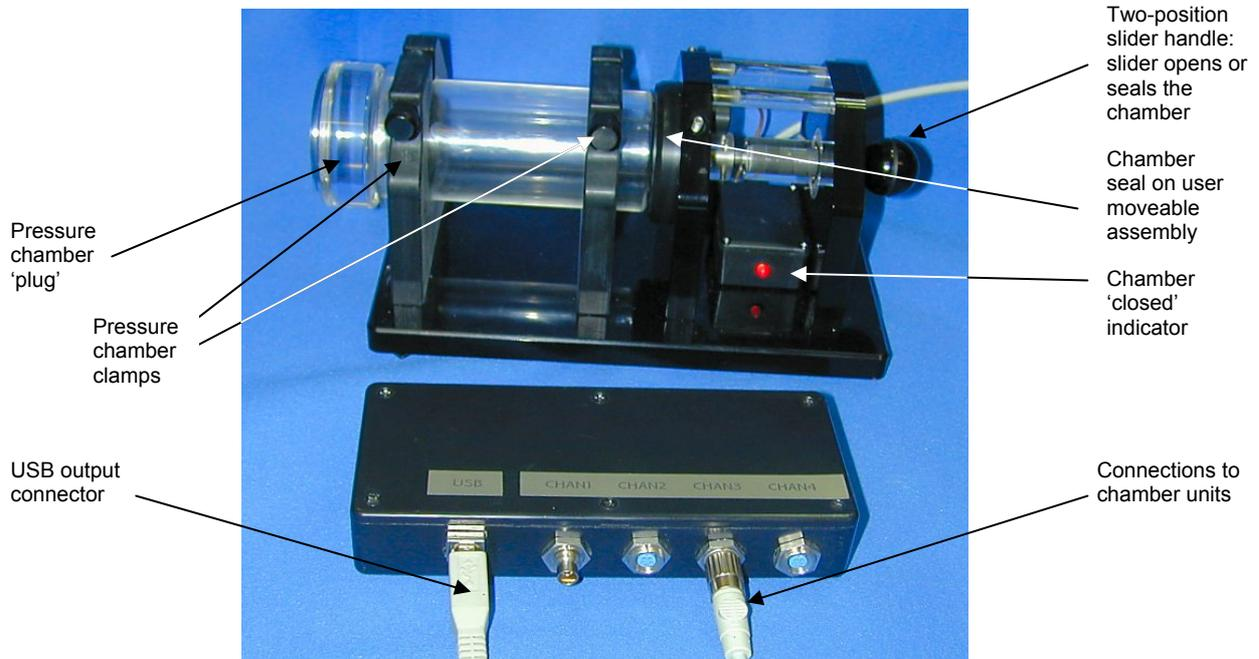
Figure 1: One of the plethysmograph chambers and the 4 channel interface unit.
