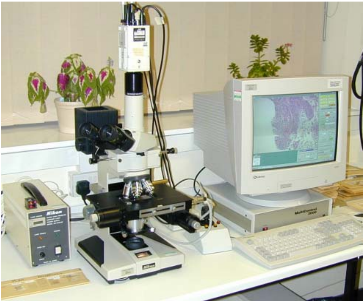
Examples of 'older' system using analogue cameras; above: system using the cooled Cohu 4900 series \frac{1}{2} " camera for fluorescence work; below: system using 3 x \frac{1}{3} " chip JVC colour camera.
