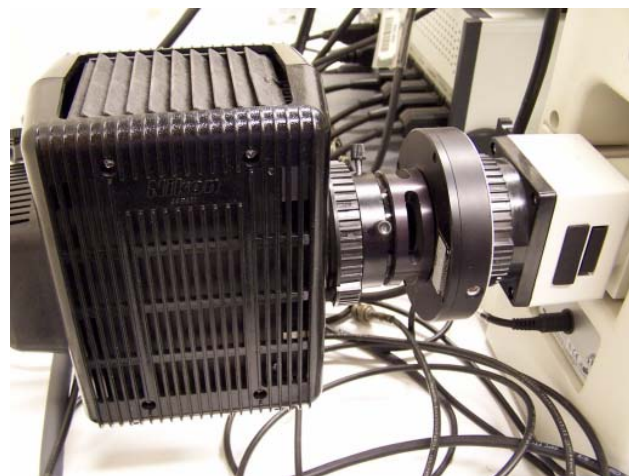
Figure 4: Fast optical shutter inserted between mercury arc lamp and microscope epi-illumination optics
