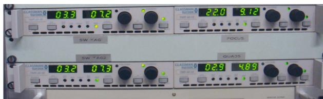
Figure 23: The external beam transport power supplies.
