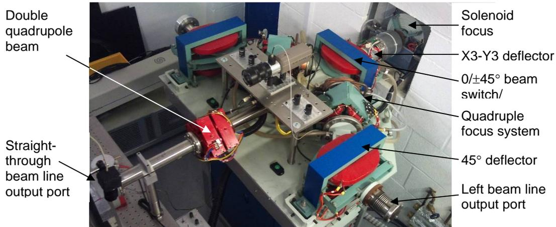
Figure 21: The linac's external beam control optics, used to shape the straight-through beam and to provide two additional orthogonal beam lines.
