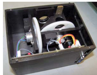
Views of rotary servo drives, used to position optical filters, mounted directly on a gearwheel, itself mounted on a rotary potentiometer acting as the feedback element
