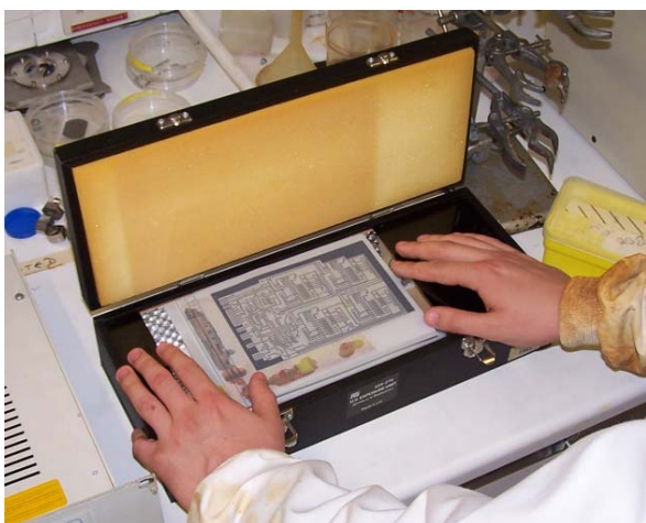
Figure 1: Preparing the artwork for exposing a double-sided board.
