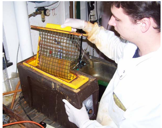
Figure 4: Etching the board.
