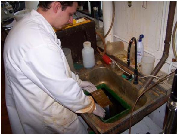
Figure 3: Developing the board.
