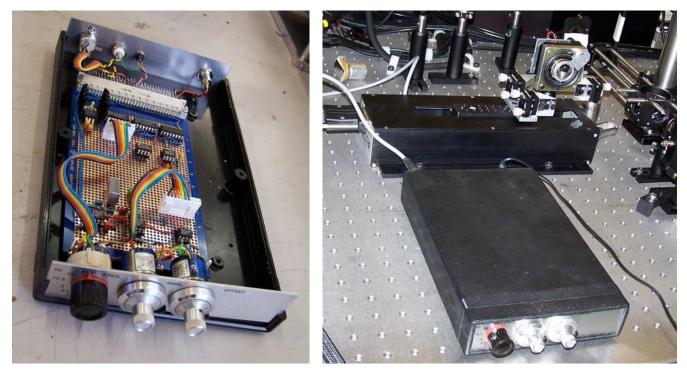
The sine-wave generator used to drive the optical delay line (left) and the complete arrangement in use (right).
