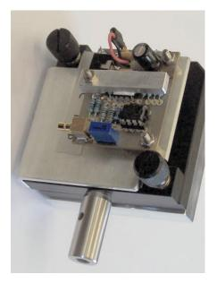
Here is an even simpler, open-loop version of the optical delay line, with just the driver and no sensor arrangement, mounted on a 2" optical mirror mount.
