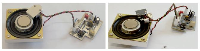
How the voice-coil optical delay line is implemented in practice: the loudspeaker and sensor assembly form a single unit which is connected to a small printed circuit board with short wires. These subassemblies are then mounted on a standard 2" optical mirror mount.
