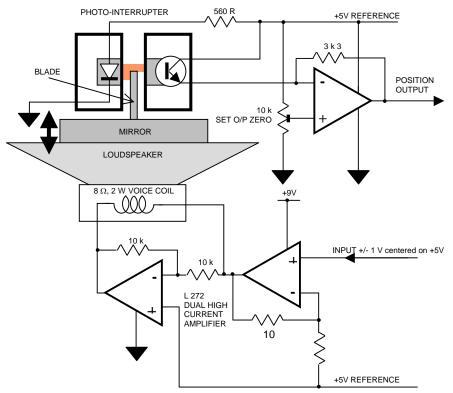
The control electronics may be modified such that the position output can be used to 'close the loop' and ensure that the loudspeaker responds to the input in a consistent, frequency independent manner. Although sinewave excitation is be primarily employed, there may be instances where other frequencies may be present, e.g. when driving the system with triangular waveforms.
