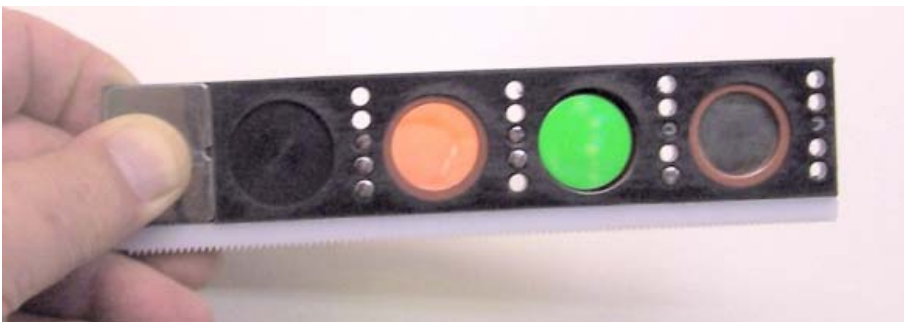
Figure 1: A version of a linear gear-driven element designed to hold 4 filters. Each element contains a set of 4 holes that are 'filled', where appropriate, with a reflective pin to generate position code with reflective sensors.
