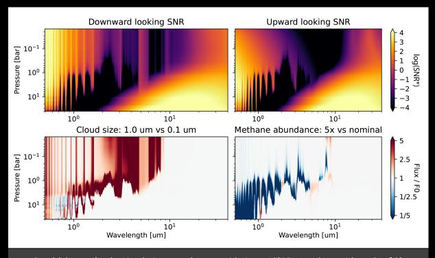
**Sensitivity study**: the simulations are done considering a 10°FOV, a solar zenith angle of 0°, emission angle of 45°, an integration time of 2-seconds, and a hypothetical filter width of 1  $\mu$ m
