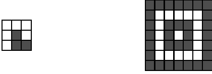
Fig. 1. (Left) Minimum number of boundary pixels in 8-neighborhood. (Right) Different levels of neighborhood system in distinct colors.
