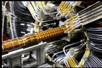
LGADs are a new development of silicon sensor technology LGADs that will increase the x-ray sensitivity (down to 250eV) and timing performance (30ps).
