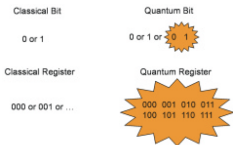
Fig. 1 A classical bit is confined to two basic states, 0 and 1, but a quantum bit (qubit) can also enter superposition states, in which the qubit is effectively in both states at once. A classical register made up of n bits can contain any one of 2^n possible numbers, while the corresponding quantum register can contain all 2^n numbers at the same time.
