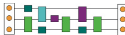
Fig. 3 Any desired quantum information processing operation can be built as a network of single qubit and two qubit gates.
