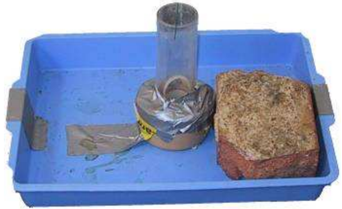
Figure 1: A photograph of the experimental apparatus. The handle of the bucket is visible at the bottom of the Perspex tube. A piece of straight wire is on top of the tube.
