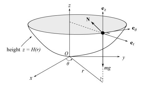
Figure 16: Particle moving under gravity on a surface of revolution.
