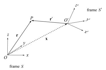
Figure 2: Relative to a choice of reference frame S, the origin O' of another reference frame S' has position vector  $\mathbf{x}$ , and the coordinate axes of S' differ from those of S by a rotation.
