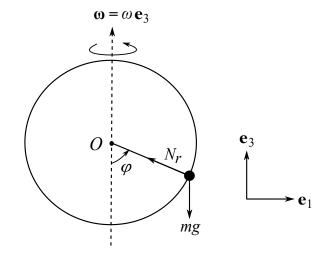
Figure 31: The bead on the rotating hoop. Here the figure shows the hoop at the instant at which it passes through the plane of the page. The component  $N_2$  of the normal reaction **N** of the hoop on the bead points into the page at this instant, which is the  $\mathbf{e}_2$  direction.
