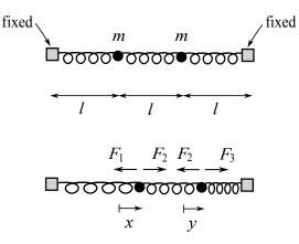
Figure 12: The system of masses and springs. The upper diagram shows the equilibrium configuration. In the lower diagram we have shown the horizontal displacements x and y of the two masses from their equilibrium positions, together with the various Hooke's law forces  $F_1$ ,  $F_2$ ,  $F_3$ acting.
