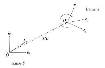
Figure 25: The reference frame  $\hat{S}$  is a fixed inertial frame. This is the frame in which we formulate Newton's laws of motion, and hence do the "observing". With respect to this frame, a general frame S has origin O at position vector  $\mathbf{x} = \mathbf{x}(t)$  as measured from  $\hat{O}$ , and its coordinate axes may be rotating, so that  $\mathbf{e}_i = \mathbf{e}_i(t)$ .
