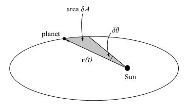
Figure 22: In a small time interval  $\delta t$  the angle subtended at the origin changes by a small amount  $\delta \theta = \dot{\theta} \, \delta t$ , sweeping out an area  $\delta A$ .
