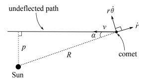
Figure 20: A comet approaching the Sun from a very large distance R with speed v. Without the effect of gravity the comet travels undeflected with constant speed v, and its closest approach is the distance p. Here  $p = R \sin \alpha$ , and the angle  $\alpha$  is very small.
