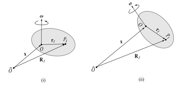
Figure 27: We fix a point O in the rigid body, which is taken to be the origin of the rest frame S of the body. The frame S has angular velocity  $\boldsymbol{\omega}$ , and its origin O has position vector  $\mathbf{x}$  relative to the origin  $\hat{O}$  of an inertial frame  $\hat{S}$ . The body particles  $P_I$  have position vectors  $\mathbf{r}_I$ , measured from O. Figures (i) and (ii) show the same body at two different times.
