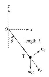
Figure 15: A simple pendulum.
