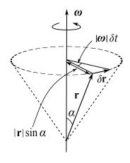
Figure 26: As seen in the inertial frame  $\hat{S}$ , the position vector  $\mathbf{r}$  of a point P fixed in the frame S changes by  $\delta \mathbf{r} = \boldsymbol{\omega} \wedge \mathbf{r} \, \delta t$  in a small time interval  $\delta t$ . This is a rotation of  $\mathbf{r}$  through an angle  $|\boldsymbol{\omega}| \delta t$  about an axis parallel to the vector  $\boldsymbol{\omega}$ . The direction of rotation is given by the right hand rule.
