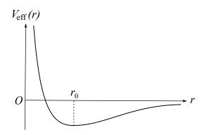
Figure 19: The effective potential  $V_{\text{eff}}(r)$  for the Kepler inverse square law force problem, crucially with  $\kappa > 0$  so that the force is attractive. In this case  $V_{\text{eff}}$  has a unique local minimum at  $r = r_0$ .
