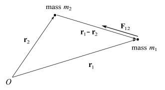
Figure 17: The attractive gravitational force  $\mathbf{F}_{12}$  on a mass  $m_1$  at position  $\mathbf{r}_1$ , due to a mass  $m_2$  at position  $\mathbf{r}_2$ . A particular physical case of interest has the Earth for mass  $m_1$  and the Sun for mass  $m_2$ .
