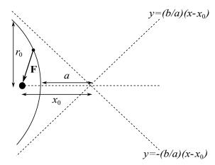
(b) A hyperbola. The large black dot is again the origin, focus, and centre of the force. The two asymptotes are  $y = \pm (b/a)(x-x_0)$ , which meet at the point  $(x_0, 0)$ , where now  $x_0 = e a > 0$ .
