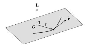
Figure 14: The planar motion of a particle acted on by a central force, with centre O. The conserved angular momentm **L** is normal to the plane of motion through O.
