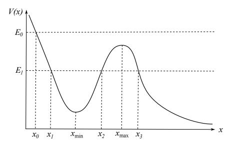
Figure 9: A general potential V(x), with various points marked on the x axis.  $x_{\min}$  and  $x_{\max}$  are a local minimum and local maximum, respectively. At any point x the force acting on the particle is minus the slope of the potential, F(x) = -V'(x).
