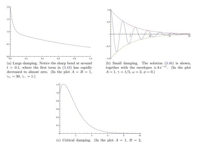
Figure 11: Various behaviours of a damped harmonic oscillator.
