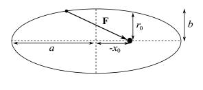
(a) An ellipse. The large black dot is the origin, which is one of the foci and also the centre of attraction (for  $\kappa > 0$ ) of the inverse square law force. The centre of the ellipse is  $(x_0, 0)$ , where  $x_0 = -ea \leq 0$ . The semi-major axis has length a, while the semi-minor axis has length  $b \leq a$ .
