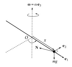
Figure 30: The bead on the rotating horizontal wire. The forces acting on the bead are  $-mg \mathbf{e}_3$  and the normal reaction **N** perpendicular to the wire.
