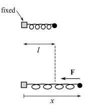
Figure 5: A spring lying along the x axis, with one end fixed at the origin. The first diagram shows the equilibrium position, while the second shows the spring extended by a length x - l > 0, with the resulting restoring force. Notice that when x - l < 0, which compresses the spring rather than stretches it, the force acts in the opposite direction (to the right).
