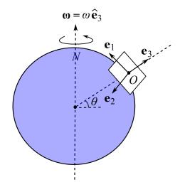
Figure 32: A frame S fixed to the surface of the rotating Earth. The angular velocity  $\omega = 2\pi$  radians per day, or  $\omega \simeq 7 \times 10^{-5}$  s<sup>-1</sup>. The latitude of the origin O of S is  $\theta$ .
