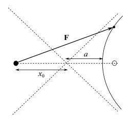
Figure 23: The other branch of the hyperbola in Figure 18b, relevant for the corresponding repulsive force. The large black dot is again the origin, focus and centre of the force.
