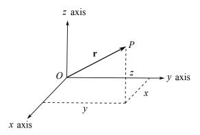
Figure 1: The position vector  $\mathbf{r} = (x, y, z)$  of a point P, as measured in a reference frame S.
