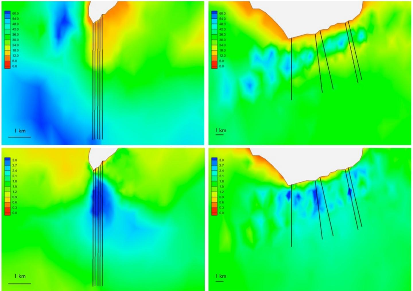
**FIGURE 4.** Locations of turbines at Portland Bill (left) and Isle of Wight (right). Top row: interpolated bathymetry (m). Bottom row: magnitude of  $M_2$  tidal current m/s. Location of turbines in this study shown with black lines. These are location 1 to 5 from left to right on Portland Bill and 6 to 10 from left to right on Isle of Wight.
