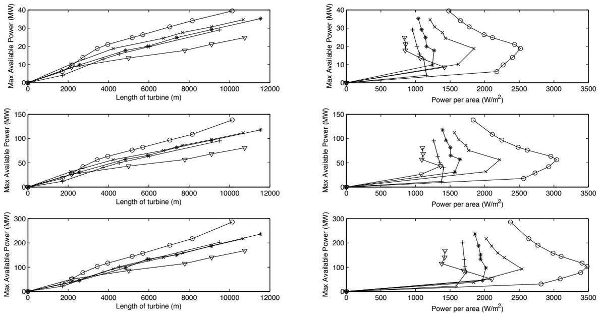
**FIGURE 7.** Results for single row of turbines at Isle of Wight. Top  $B = 0.1$ ; middle  $B = 0.25$ ; bottom  $B = 0.4$ . Left: length of turbine array against maximum available power; right: power per swept area vs available power. Symbols indicated location of turbines: ‘+’ – location 6; ‘o’ – location 7; ‘\*’ – location 8; ‘x’ – location 9; ‘∇’ – location 10.
