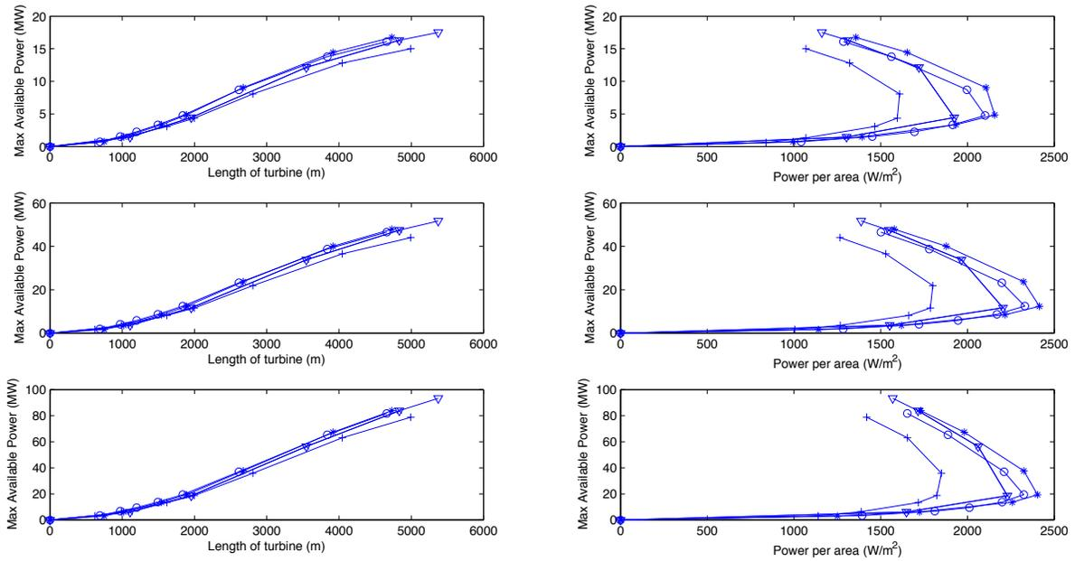
**FIGURE 5.** Results for single row of turbines at Portland Bill. Top  $B = 0.1$ ; middle  $B = 0.25$ ; bottom  $B = 0.4$ . Left: length of turbine array against maximum available power; right: power per swept area vs available power. Symbols indicate position of turbines: '+' – location 1; 'o' – location 2; \* – location 3; × – location 4; ∇ – location 5.
