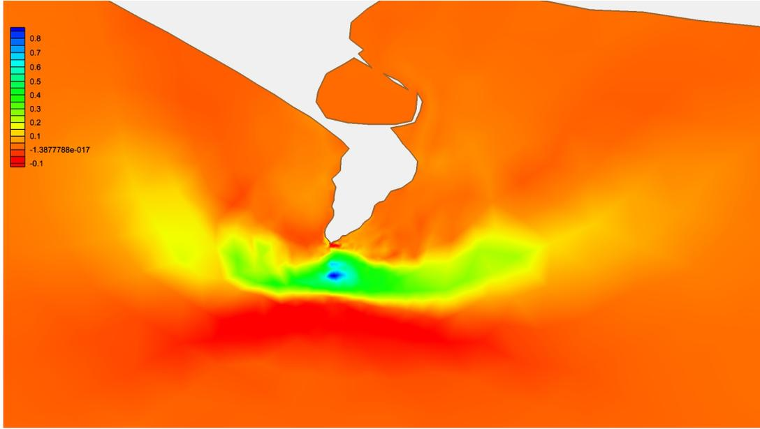
**FIGURE 8.** Magnitude of the change in the  $M_2$  tidal current around Portland Bill between undisturbed flow and an array of turbines extending 2.7km offshore with  $B = 0.4$  operating at the point which gives maximum available energy.
