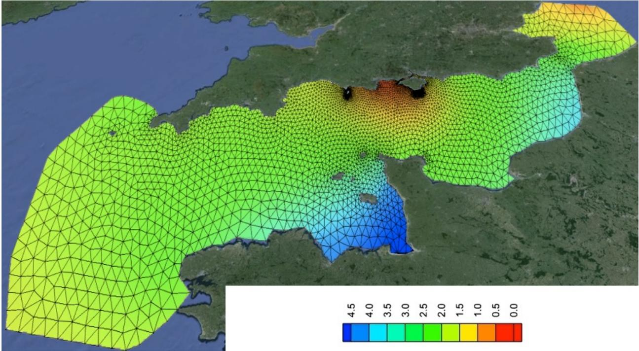
**FIGURE 1.** Numerical mesh used in study shown in Google Earth. Colours indicate the modelled  $M_2$  water level amplitude in m.
