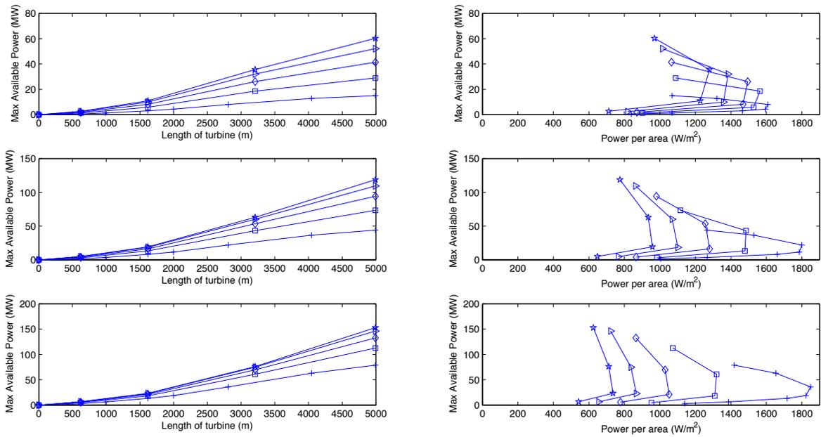
**FIGURE 6.** Results for multiple rows of turbines at Portland Bill. Top  $B = 0.1$ ; middle  $B = 0.25$ ; bottom  $B = 0.4$ . Left: length of turbine array against maximum available power; right: power per swept area vs available power. Symbols indicate number of turbine rows: + – one row; square – two rows; ◇ – three rows; △ – four rows; \* – five rows.
